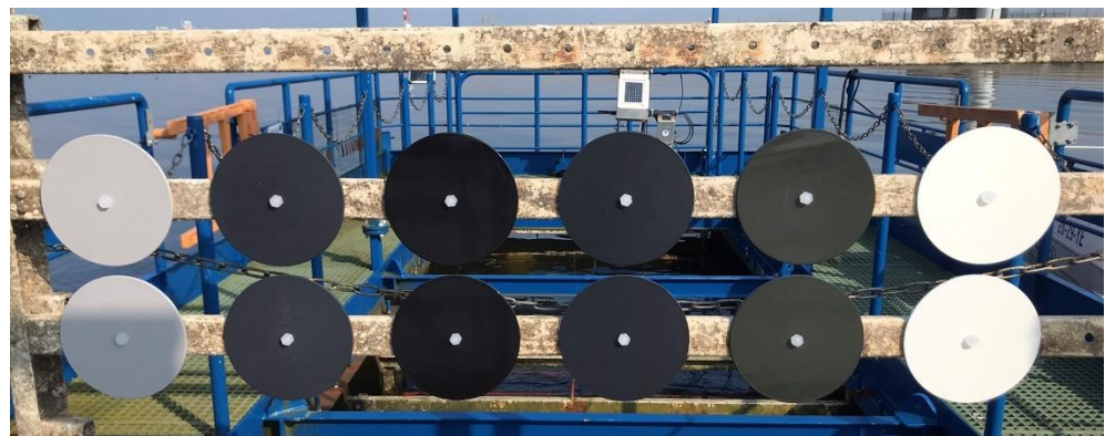
Figure 2: Disc placement during the raft exposure before immersion for the ‘static’ exposure tests and subsequent FDM measurements – from left to right: Intersleek, Jotun, Hempablue, Trilux, Hempaguard. Two replicas of each coating are stacked vertically and denoted as R1 (top) and R2 (bottom). The front of the discs are pictured.
